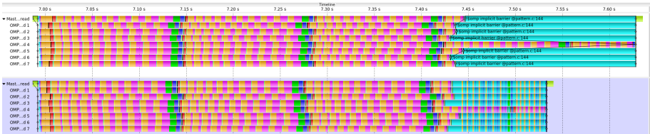
Fig. 2. Trace comparison of our reference GMRES kernel (top) and the conditional nested tasks version (bottom) both using 8 OpenMP threads.
